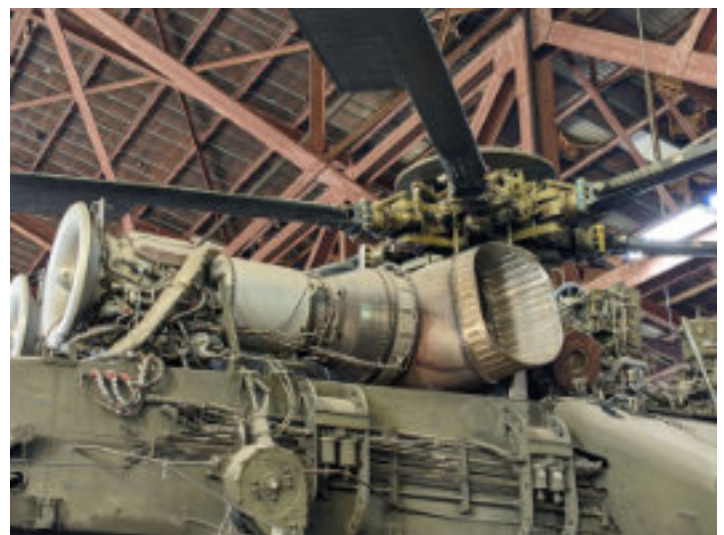
CH-54 engine and rotor head (K. Drewelow photo)
